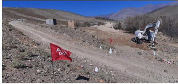
ATC Hitachi Demining Machine Clears an AV minefield that had blocked a road and residential area in Chak
